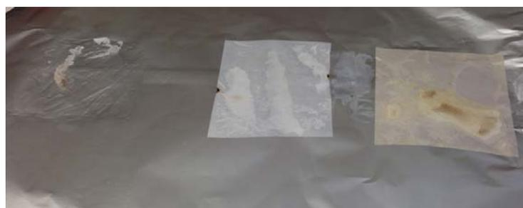
Figure 9: Photo of tri-layer, Dreamweaver Silver and Dreamweaver Gold separators after having been engulfed in flaming electrolyte.
