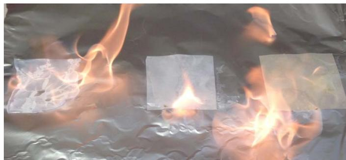
Figure 6: Photo of tri-layer, Dreamweaver Silver and Dreamweaver Gold separators that have been saturated in electrolyte and then lit on fire.
