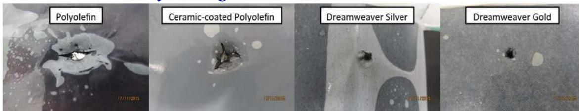
A team of investigators led by Dreamweaver International has investigated the effects of heat and nail penetration on lithium ion cells by performing autopsies on cells post-test.
